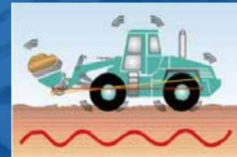
The hydraulic joystick integrated with the FNR switch realizes the rapid switching of the machine forward and reverse, and improves the work efficiency.
