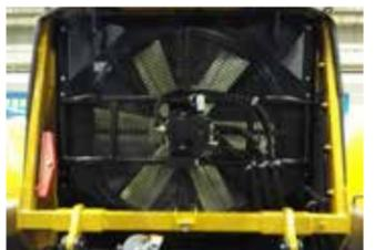
Intelligent independent cooling system, automatic and stepless adjustment of fan speed, reduce operating noise, and can significantly reduce fuel consumption.
