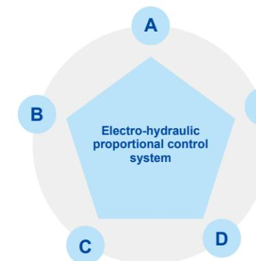
**A** Buffering function: When the boom is activated, stopped or close to the limit, the action buffer is decelerated to prevent impact and avoid severe vibration.
